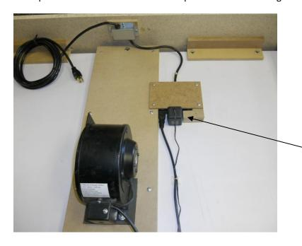
The plug from the blower motor and the AC Adapter should be plugged into the power strip mounted on the underside of the table. Use the wire ties to help secure the cables to the bottom of the table.
