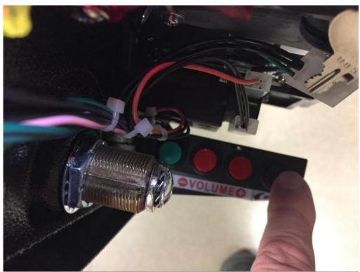
3. "DIAG" will be highlighted, Press the menu button again to enter the Switch Test menu.
