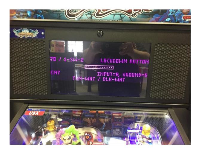
7. Press the lockdown Switch while observing the screen, you should hear a ding, a box should appear on the left side of the center bar and the brightness of the menu will change.
