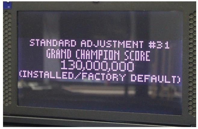
7. Press 'Menu' button to enter setting. Use Volume +/- to adjust score. Press 'Service/Credit' button to exit setting.
