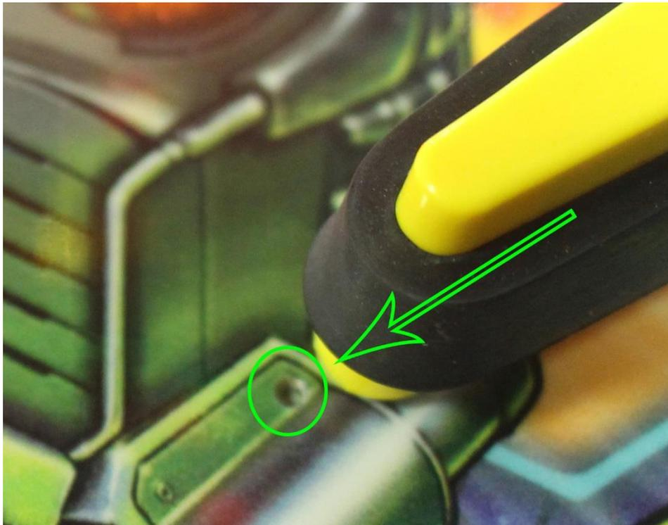
10. Tighten the crank arm screw.
