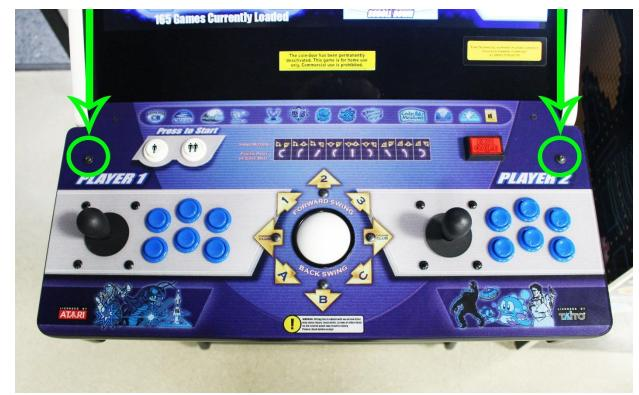
2. Using a Phillips head screwdriver, loosen both screws until they come all the way out of the control panel. Set screws aside in a secure location.
